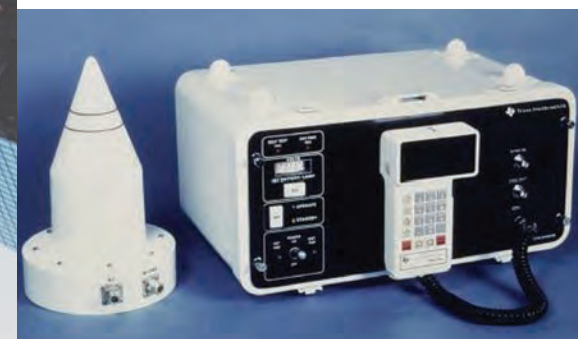
A TI4100 GPS receiver developed and built by Texas Instruments in the early 1980s, the first field-deployable GPS receiver on the market. Calgary-based Nortech Surveys ordered the first four commercial units produced in 1981 and used them to successfully conduct surveys around the world for the ocean-exploration and energy industries until the late 1980s.
