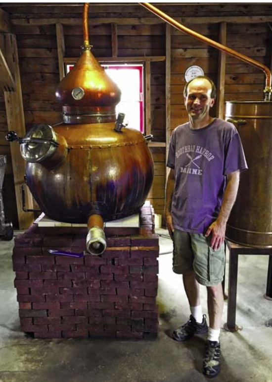
Bodine stands next to his alembic pot still. Steam from the boiling molasses goes through the overhead line and cools down in the container at right.
