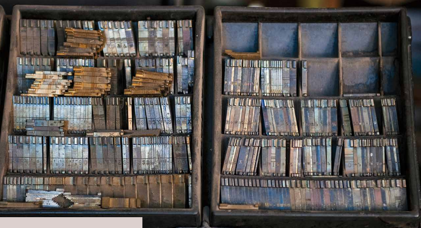
Linotype matrices – tiny molds for casting lines of lead type – fill racks at the office of The Saguache Crescent , the last newspaper that still uses Linotype. Editor Dean Coombs uses the same equipment his grandparents bought in 1921.
