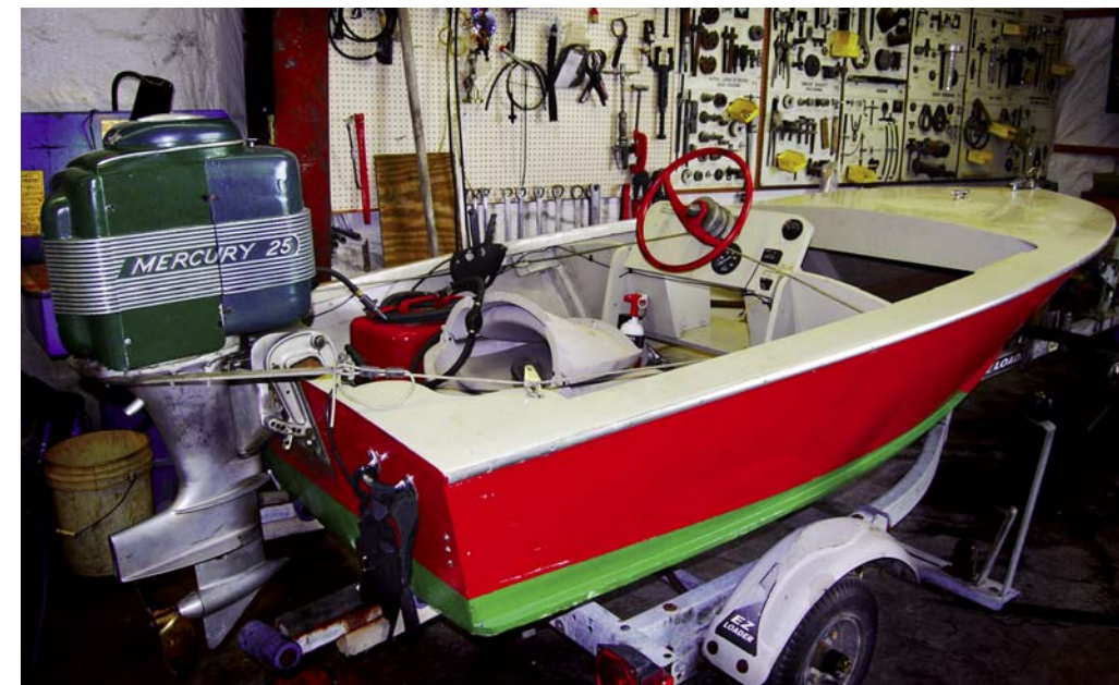
Davis and his son, Andrew, built this PB4, a Custom Craft kit boat, in the 1990s. The engine is a 1950 KG9 Mercury 25 HP with a Quicksilver leg and 1:1 lower unit for racers.
