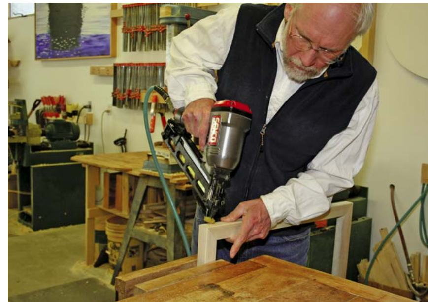
Framer Chris Polson uses a pneumatic nailer to assemble a stretcher.
