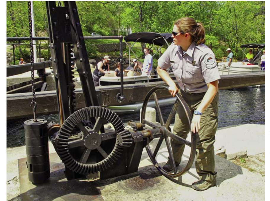
State Park Ranger Lauren Hillier operates the antique sluice gears at Songo Lock.
