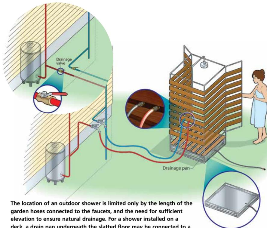
The location of an outdoor shower is limited only by the length of the garden hoses connected to the faucets, and the need for sufficient elevation to ensure natural drainage. For a shower installed on a deck, a drain pan underneath the slatted floor may be connected to a hose to direct waste water away.
